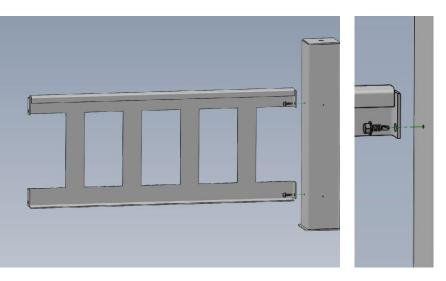
USING TWO SCREWS, ATTACH THE FOUR SIDES TO THE FOUR LEGS. TO MAKE IT EASIER FOR YOU, YOU CAN PRE-DRILL WITH THE SELF-DRILLING SCREWS BEFORE ASSEMBLY.
